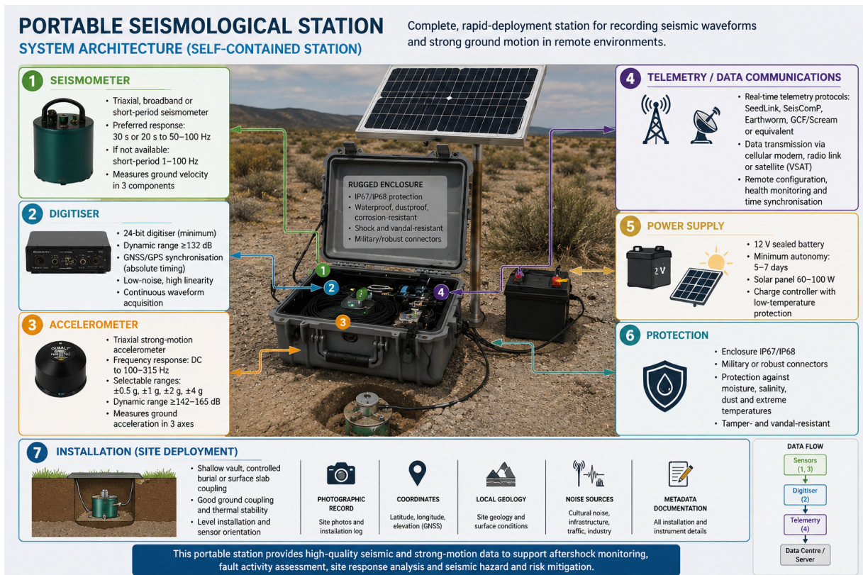
Figure 2 Architecture of a self-contained portable seismological station system
